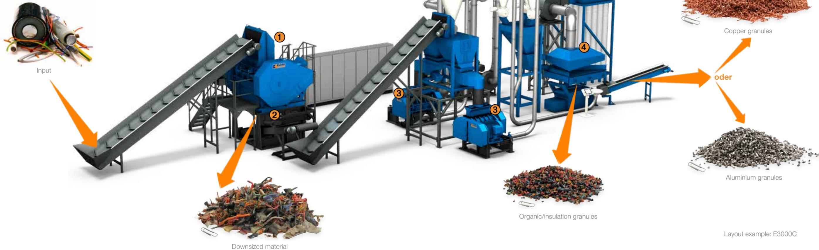
**1. ELDAN Multi Purpose Rasper.** This machine is an effective, medium-speed, dual drive Rasper designed for cable recycling. It ensures individual size reduction down to approx. 15-25 mm fraction sizes.
